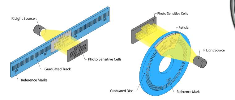
An encoder's most important components include a light source, scanning reticle, gratings, and a photosensitive sensor. The gratings can be arranged in a circular shape—for example, angle and rotary encoders—or along straight path in linear encoders. Typically, the scanning reticle and grating used in an encoder are matched to have equal periods.
