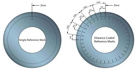
using a certain mathematical algorithm, typically with distance between each set of marks progressively decreasing by 1 grating period. This allows reestablishment of the absolute position with only minimal movement. Distance-coded reference marks are extensively used on both linear and angle encoders.
