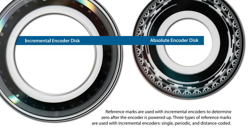
In case of single marks, entire encoder has just one mark, and exact zero can be established by monitoring reference output after crossing the mark. Single marks are commonly used on rotary encoders. However, they can be disadvantageous when used on linear encoders, since a long distance must be traveled before zero is established.
